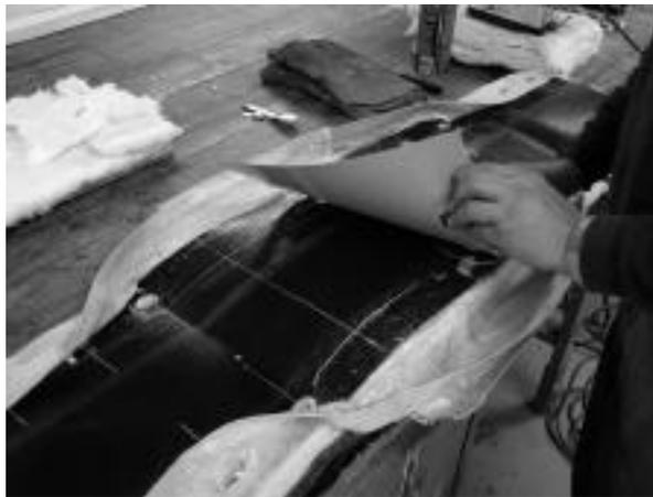
Figure – 9 Overlap inner fiberglass layer.
