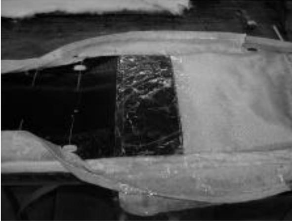
Figure 10 – Position PFA adhesive film
