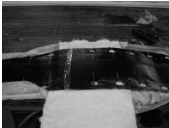
Figure 12 – Position insulation covered plywood board.
